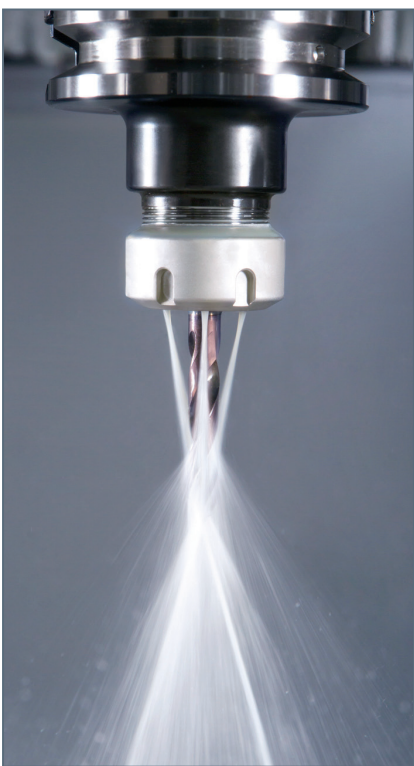
Seal Jet With angular nozzles. Coolant flow is direct to the cutting edge - for use with standard straight shank cutting tools (without coolant hole).
